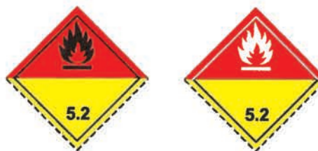
Symbol (flame): black or white; Background: upper half red; lower half yellow; Figure '5.2' in bottom corner
